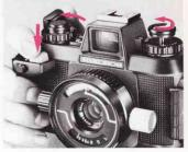
**18.** Make blank exposures until the frame counter shows "4"
